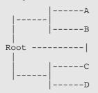
The topology of this dendrogram tells us a simple story: It says that A and B are more similar to each other than they are to C and D. Thus if we align A with B, we are less likely to make a mistake than if we align A with C or D.
